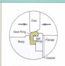
The metal seat ring allows control of extremely hightemperature fluids, and replaces conventional gate valves, globe valves, and ball valves. (eg. steam, compressed air, combustion gas, exhaust gas, sulfurous-asid gas, nitrogen gas)
