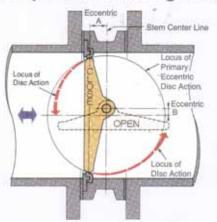
Since the stem is eccentric from the seat ring (as indicated by A and B), the disc is in contact with the seat ring only when the valve is completely closed. The benefits from the double eccentric disc design include:
