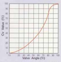
\* The chart shows the flow characteristics curve at 200 mm size (8').
