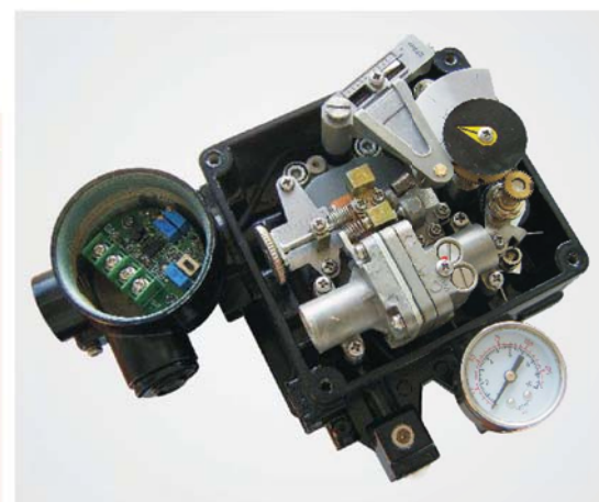
positioner with position transmitter
